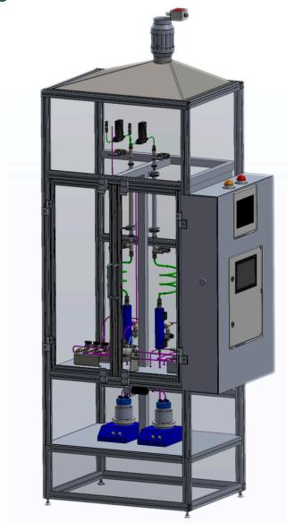
Our integrated H<sub>2</sub>-warning system will give an alert signal, once a critical hydrogen level is reached inducing a safe shut down process.
